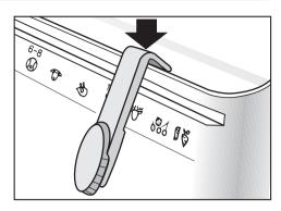
■ Clip the markers over the guides at an angle of approx. 45°. Press downwards until they click into position.
